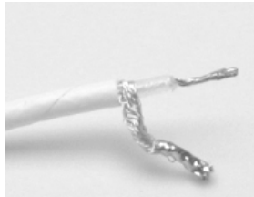
Poor Coax Preparation
